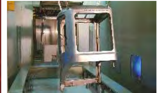
KTL-Grundierungen bieten optimalen Korrosionsschutz. Cathodic dip coating offers optimal protection against corrosion.
