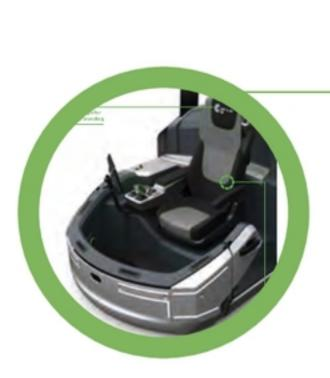
Grammer provides an ergonomically optimized complete seating system, which comprises a suspended operator's seat featuring electrically configurable features, multifunctional armrest and 12in multitouch display designed in association with Dresden University of Technology (for more details see page 111)
